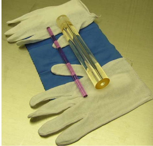
Figure 1.1 Example of a rod-in-tube phosphate glass preform with Nd-doped core rod.
