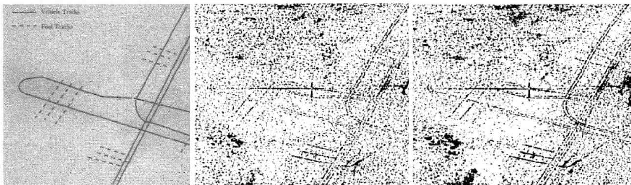
Figure 7. X-band ground truth, HH, and fully polarimetric coherent change detection comparison of man-made tracks (from left to right), showing improved observation. 6
