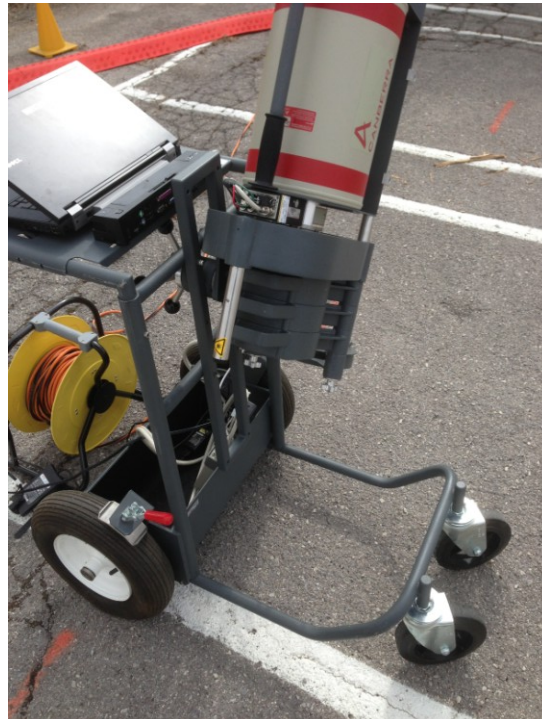
Figure 9. ISOCS measurement of asphalt at test bed.
