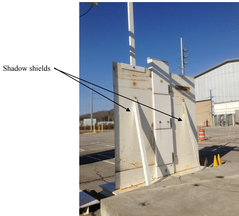
Figure 4. Custom-built shadow shields shown on one RPM pillar.
