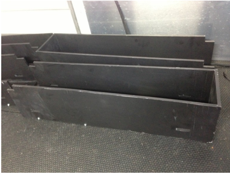
Figure 3. TSA Systems lead collimators.
