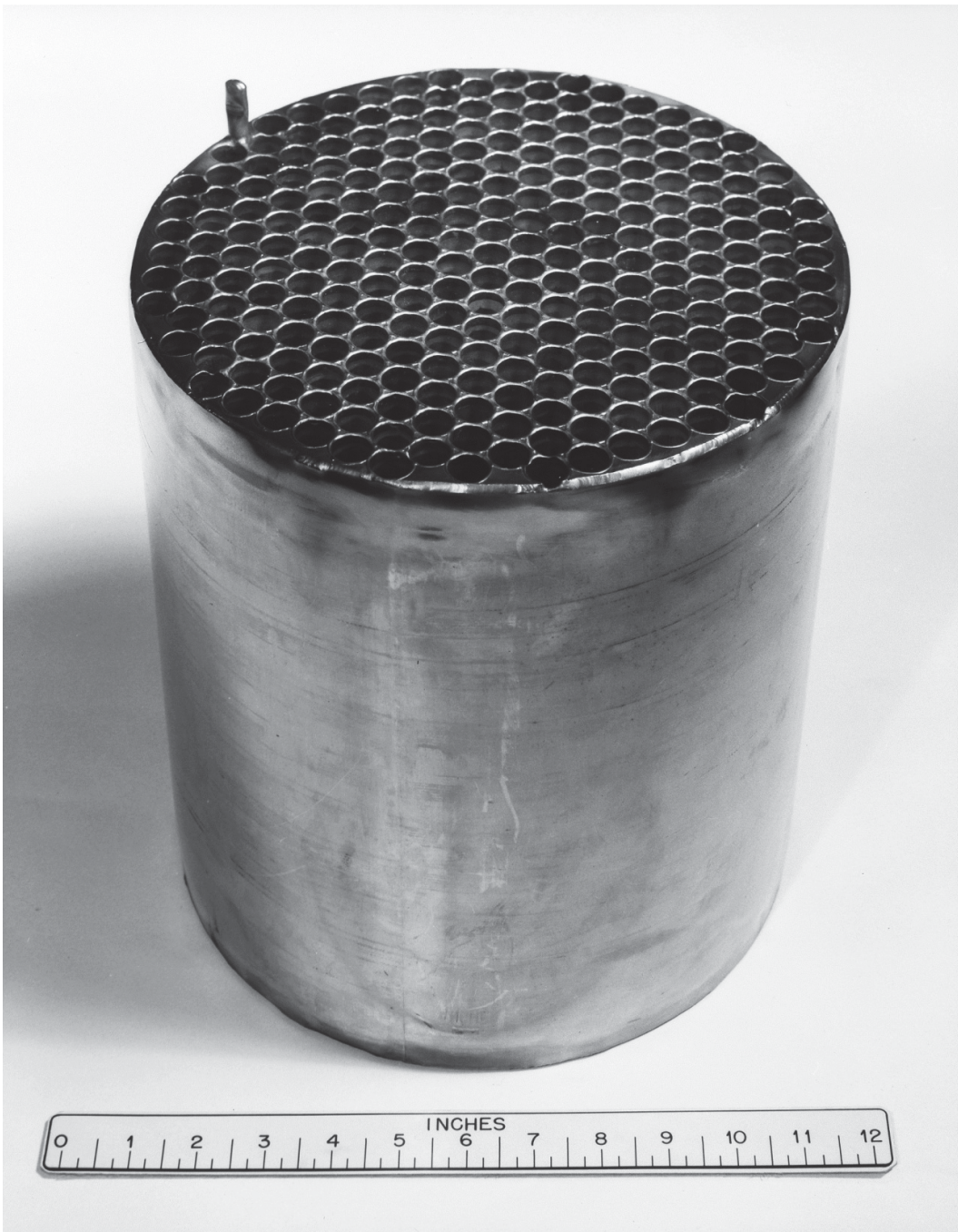
Figure 1.4-4. Potassium Filled Calandria (see Reference 4). b
