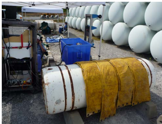
Figure 4.3. A typical measurement configuration. The 30B cylinder is covered with lead blankets to reduce the gamma-ray contamination in the EJ-309 scintillator cells. The detectors are arranged in the blue box. The electronics rack is in the vertical crate seen on the left.
