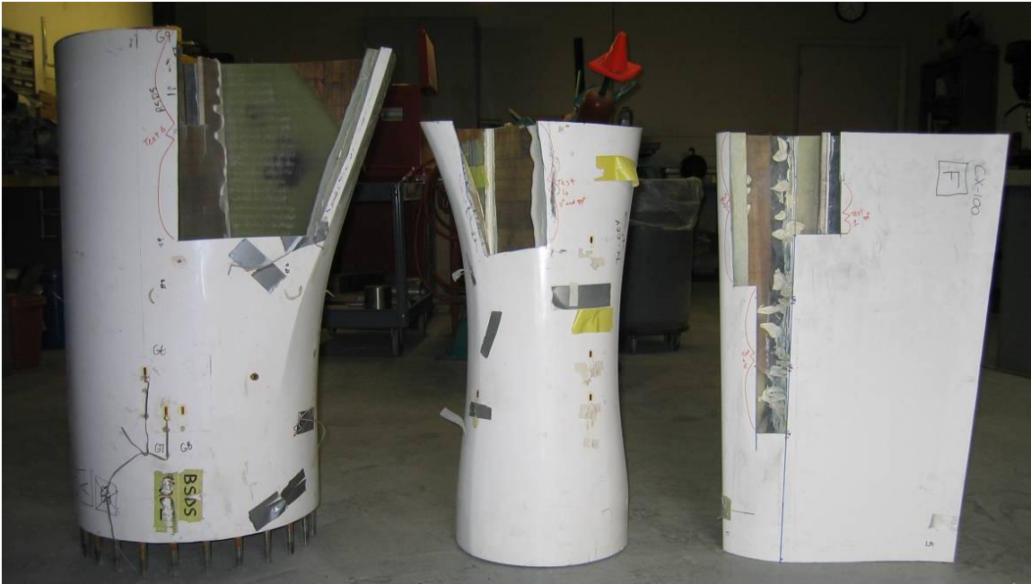
Figure 9: Blade sections after removing samples. From left to right: BSDS, TX-100 and CX-100 blades.
