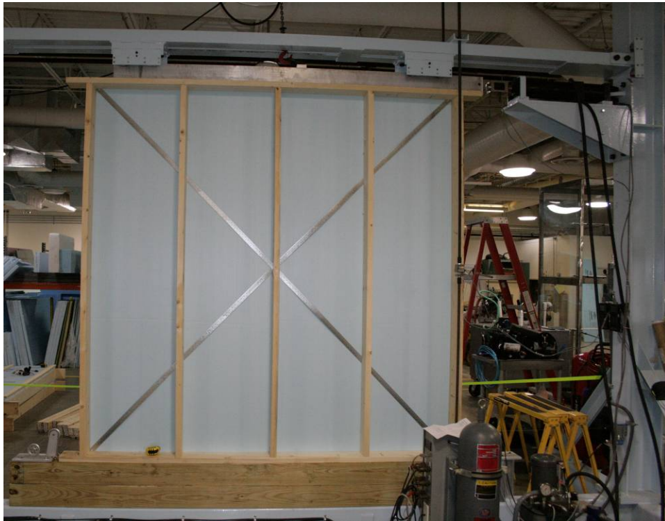
Figure 20. Structural test wall 1 installed in apparatus
