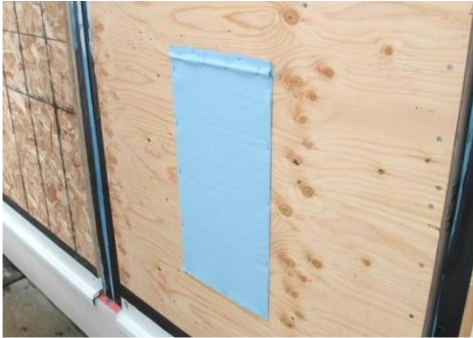
Figure 27. Exterior wetting apparatus
