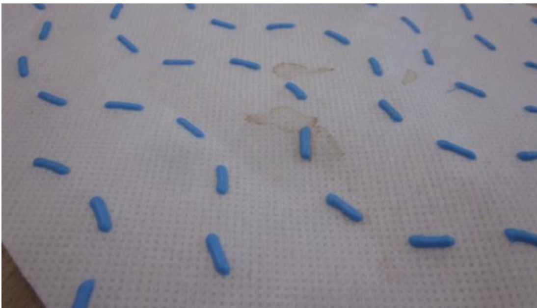
Figure 19. Example of a bumpy housewrap
