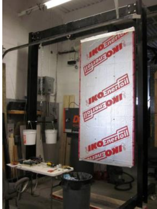
Figure 4. Drainage and drying balance
