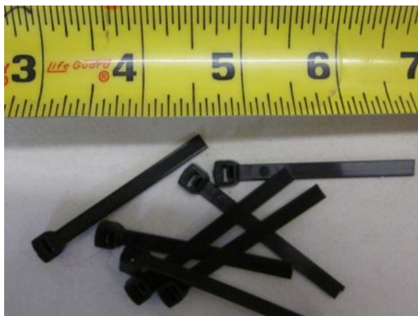
Figure 10. Two-inch-long plastic spacers
