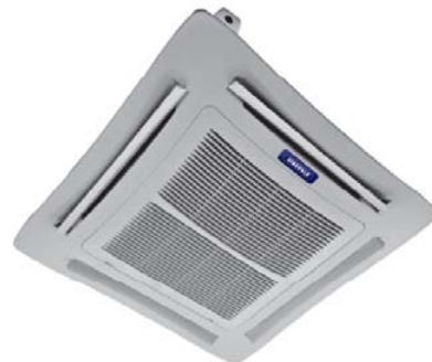
Figure 4. Airedale's cassette is ceiling mounted and integrates fan, coil, and supply and return grilles in a single package
