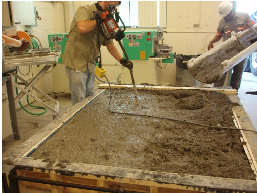
Fig. 13. Consolidating the specimen with an internal vibrator.
