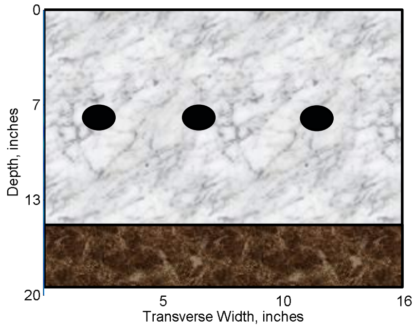
Fig. 81. Schematic of the CRCP subsurface at the example scan location.
