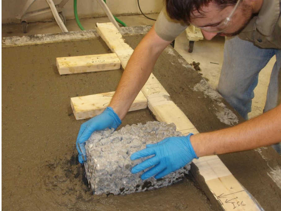
Fig. 14. Installing the surface level pervious concrete prism. Note the long guide board use to align the surface defects and the two short boards holding the triangular plates used to simulate cracks.
