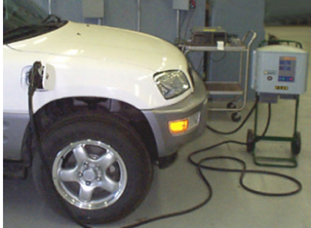
Figure 5.25: Toyota RAV4 EV charging with a conductive charger inside the vehicle (EVSE is also shown outside the vehicle here) [18].
