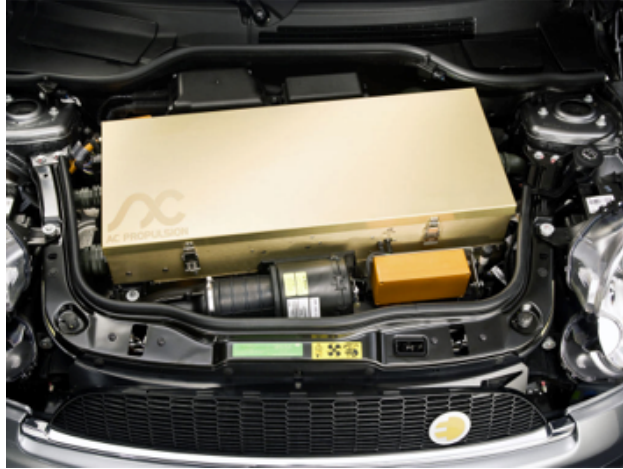
Figure 5.2: AC Propulsion integrated charger under the hood (Photo credit: BMW).
