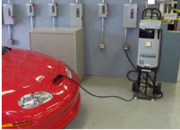
Figure 5.11: 6.6 kW external inductive charger of GM EV1 [14].
