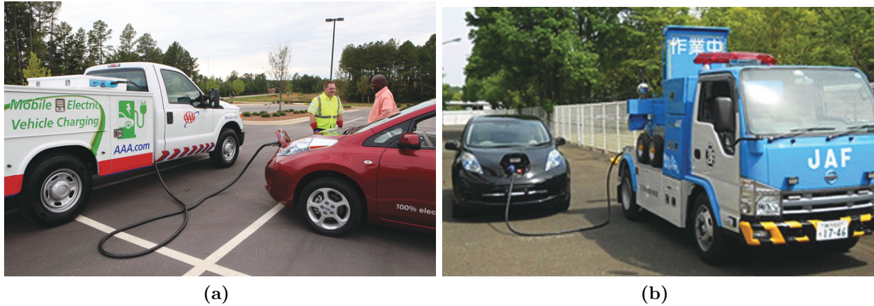
Figure 3.5: (a) AAA emergency charging service [11] and (b) Nissan mobile EV charging vehicle [12].
