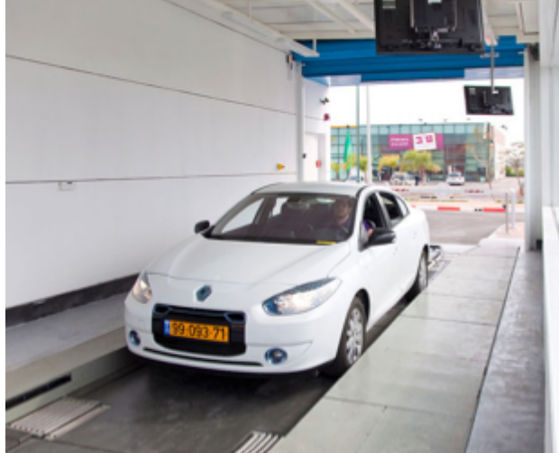
Figure 5.16: Renault Fluence Z.E. ready to switch its battery pack (Photo credit: Project Better Place).
