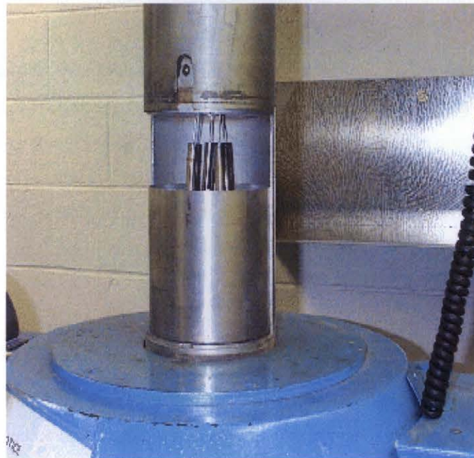
Fig. 3.2. Irradiation chamber of ORNL ^{60}\text{Co} irradiator with sample containers installed.
