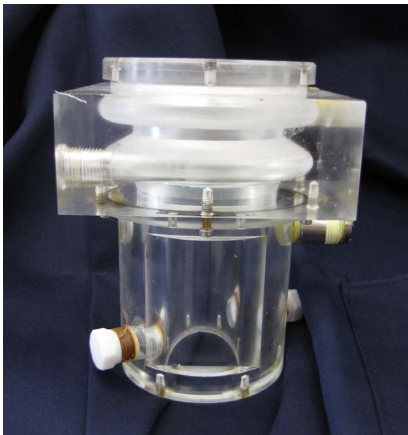
Fig. 10.1. Transparent housing based on CINC model V-2 contactor.
