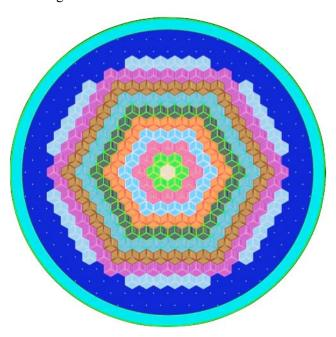
Fig. 11. AHTR core model for power distribution calculations.
