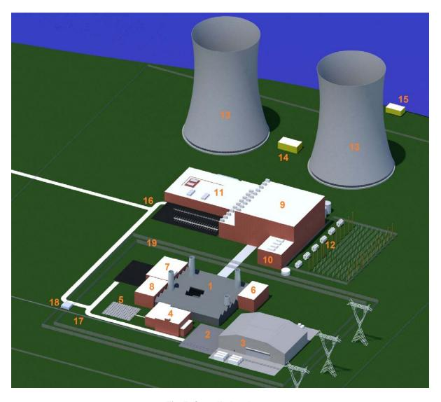
Fig. 7. Overall plant layout.
