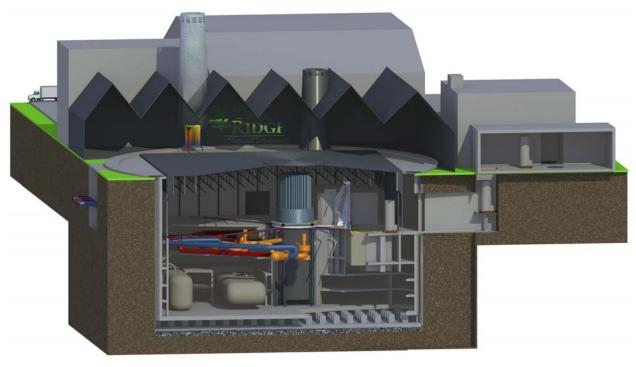
Fig. 5. Overall depiction of the reactor block features.
