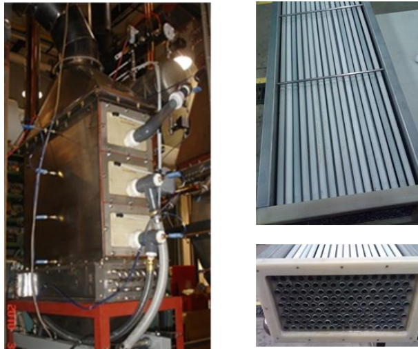
Figure 60. (left) prototype TMC test system used for evaluating metallic-substrate tubes and (right) front and top view of metallic-tubes module
