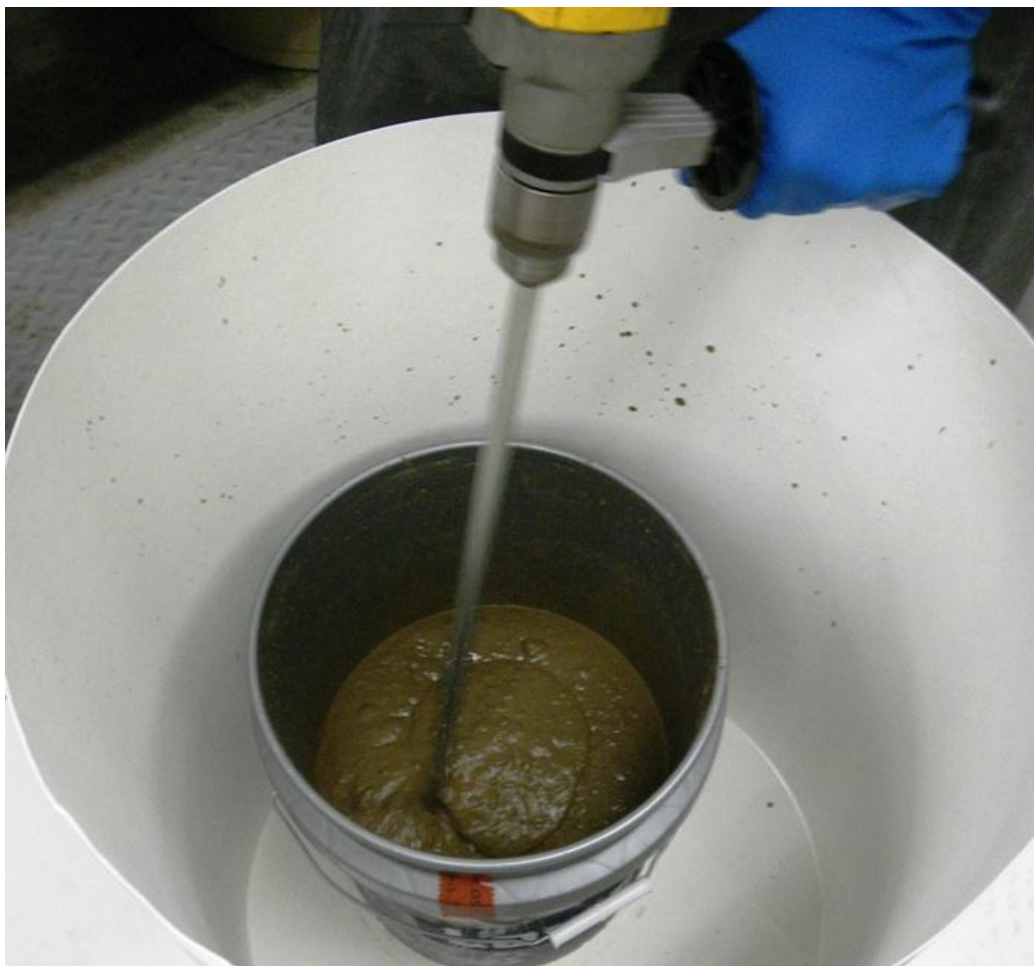
Figure 2. Sediment sample from the lower Emory River being mixed at ORNL with a customized stainless steel bit attached to a variable-speed drill.
