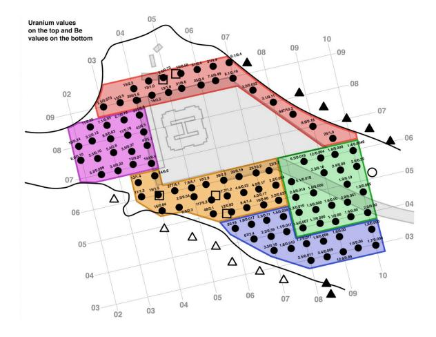
**Figure 3.** The location of soil samples collected from the berm of the AHW crater.
