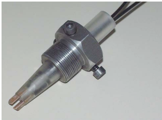
Figure 3. Photograph of the in-flow conductivity sensor.
