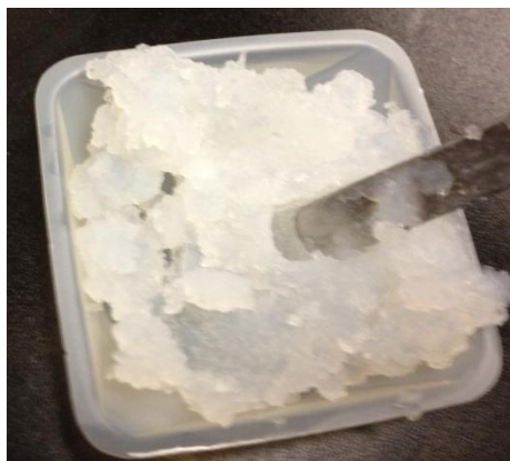
FIGURE 12. DUCTILE PASTE FORMED IN THE TRANSITION BETWEEN GELATION AND NON-GELATION REGIMES.
