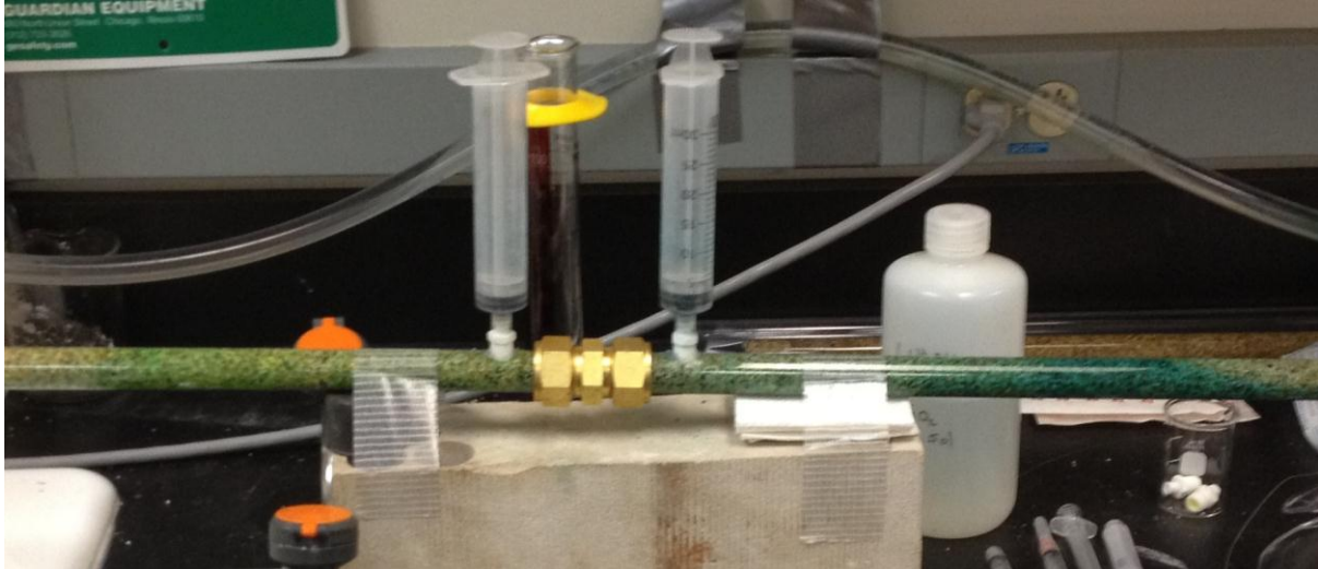
FIGURE 16. CLOSEUP OF FIGURE 15. ISOLATED CIRCULATION CELL IN POROUS MEDIA. SILICA GEL IS DYED GREEN (ON THE LEFT) AND BLUE (ON THE RIGHT) TO INDICATE LOCATION OF BLOCKAGES. THE INJECTION AND PRODUCTION WELLS ARE STILL ABLE TO COMMUNICATE WITH EACH OTHER.
