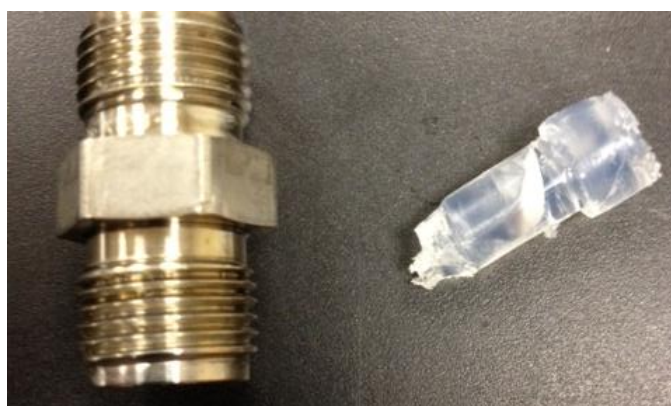
FIGURE 8. GEL (RIGHT) PRODUCED IN A 300 °C OVEN. WATER WAS PREVENTED FROM ESCAPING BY SEALING THE COLLOIDAL SOLUTION IN A SWAGELOK CAPSULE (LEFT). THE SHAPE OF THE GEL REFLECTS THE INTERNAL GEOMETRY OF THE CAPSULE.
