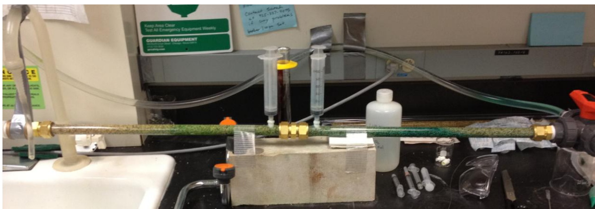
FIGURE 15. FLOW-THROUGH APPARATUS TO OBSERVE FLUID DIVERSION IN POROUS MEDIA
