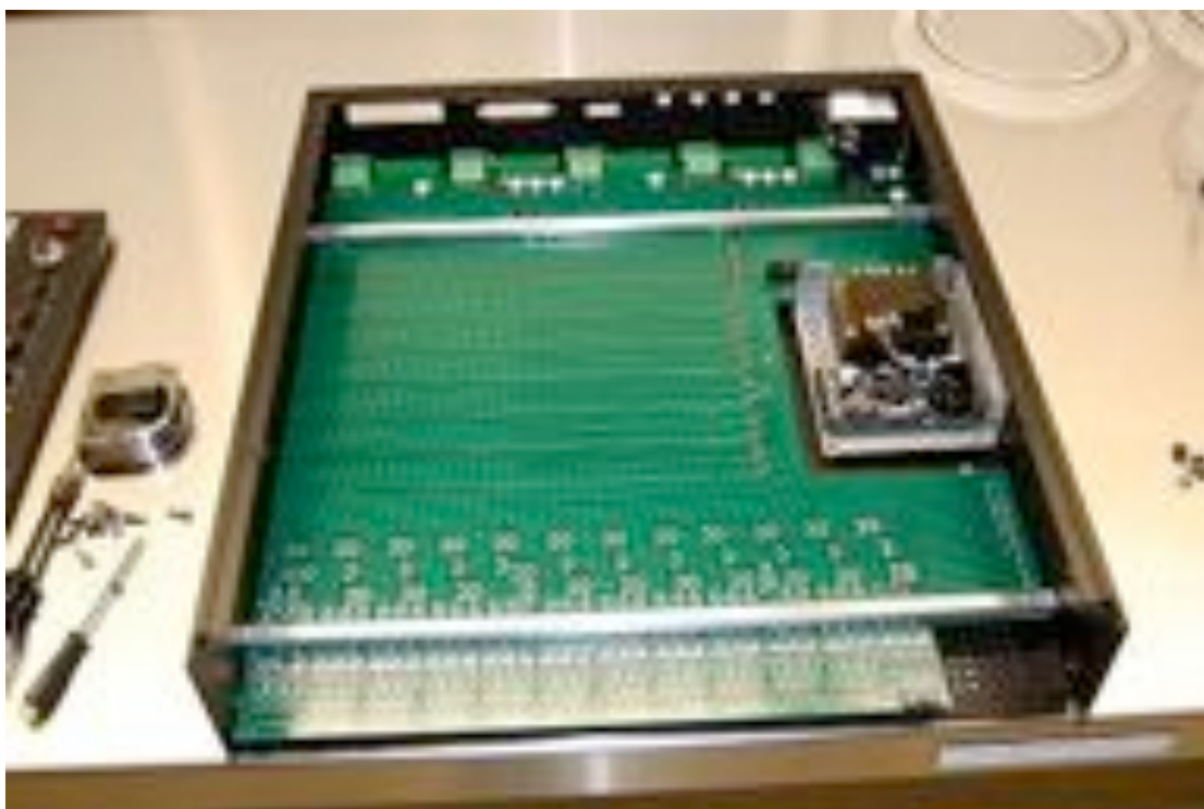
Figure 6: One of two PCBs that make up the power distribution rack. The lower PCB shown here which controls the analog is ready for testing. The upper PCB (not shown) is also complete and mounts above this board in the same rack.
