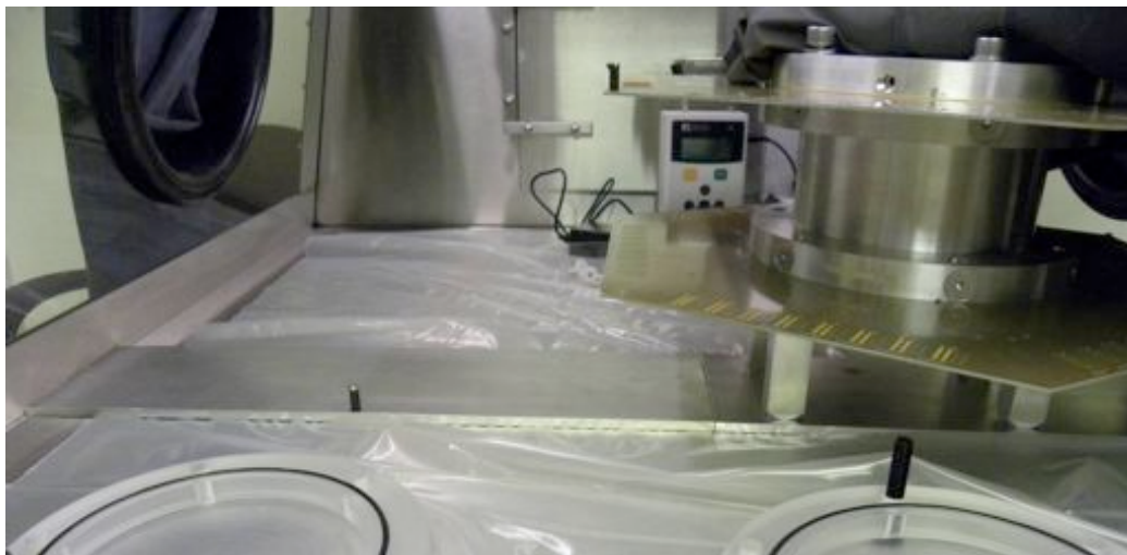
Figure 38: Stand to securely hold TPC in glove box.
