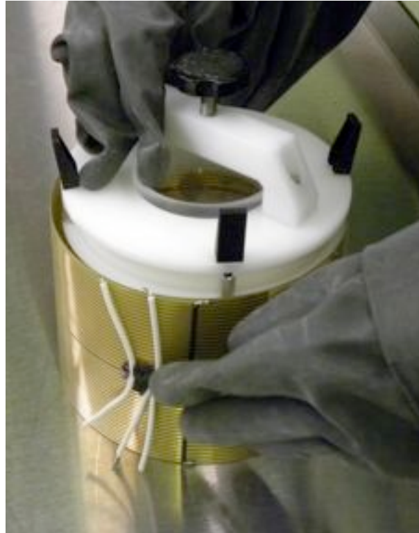
Figure 37: Top cap to seal radioactive samples into field cage.
