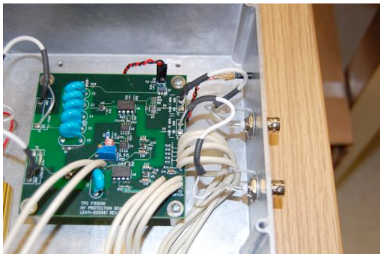
Figure 2: New high voltage system for the micromegas.
