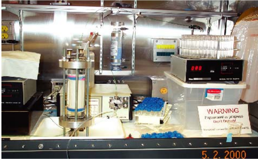
Figure 2.1 Photograph of experimental set-up showing membrane sealed core in flowthrough reactor. Gradient HPLC pump that controlled flow rate is behind the flowthrough reactor, and the fraction collector for outflow solutions is seen at right.
