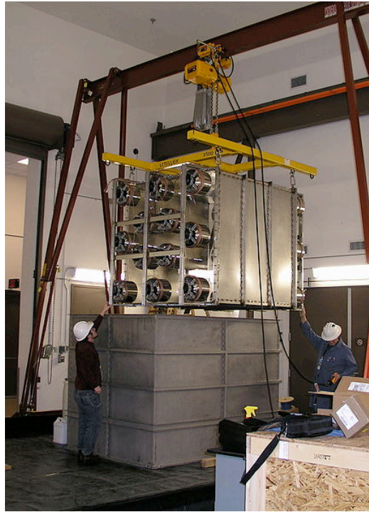
Figure 3. Assembly of the inner detector volume.
