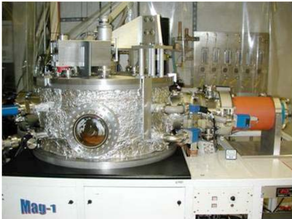
Figure 6. The Mag-1 magnetron sputtering system was used to deposit the SiO 2 -Cu-SiC coatings on ZnSe and ZnS discs
