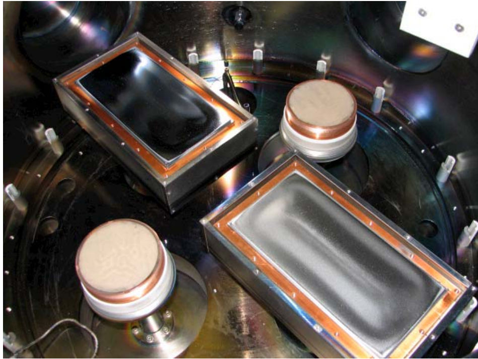
Figure 7. Two sputter targets inside the Mag 1 chamber
