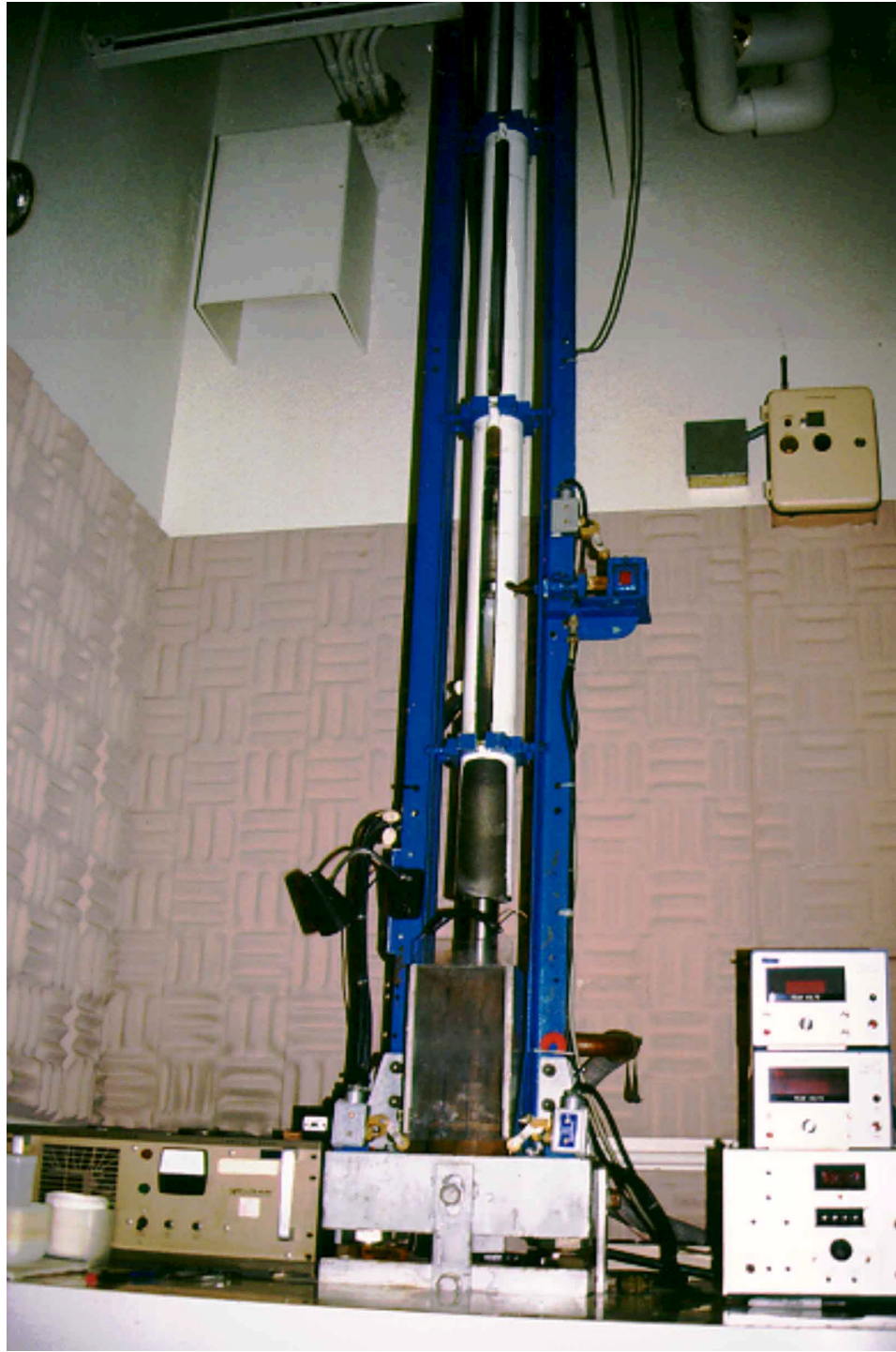
Figure 1. Drop hammer system at LLNL
