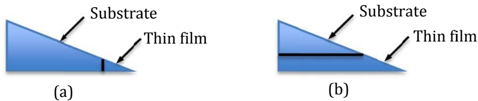
Figure 1.11 Schematic drawings of thin areas in (a) cross-section and (b) plan-view TEM specimens after ion milling.
