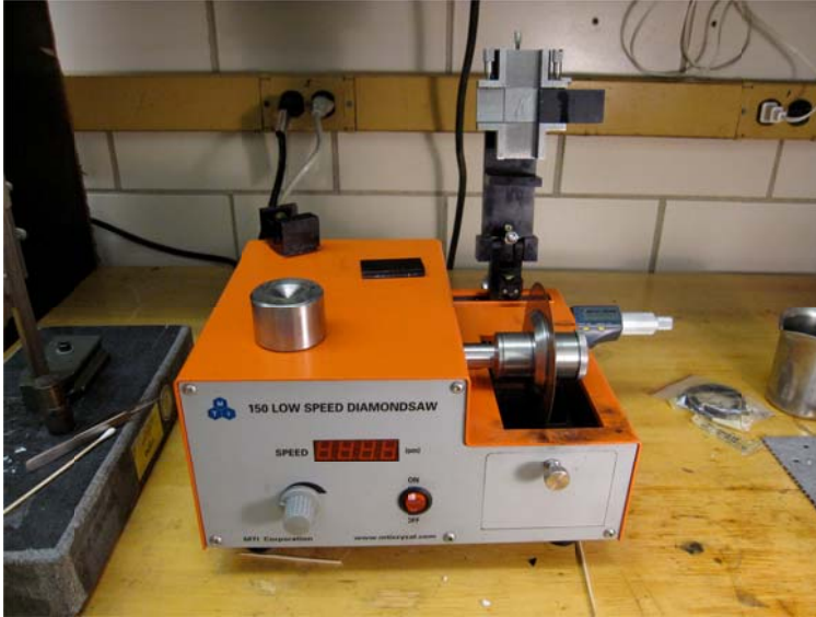
Figure 1.5 Low speed diamond saw located in Materials Research Laboratory at the University of Illinois
