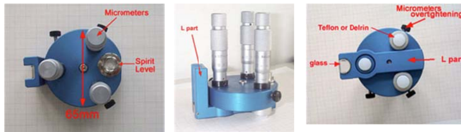
Figure 1.7 The top, side and bottom view of a tripod specimen holder
