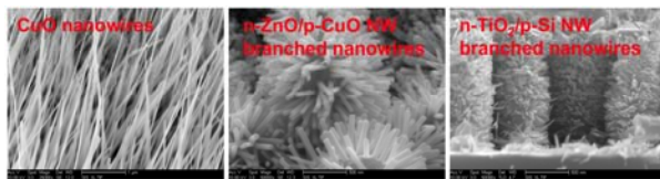
Figure 18. Future works on other nanowire PEC devices consists of CuO nanowires, 3D branched ZnO/CuO, and TiO 2 /Si branched nanowire photoelectrodes for high efficiency of better stability.
