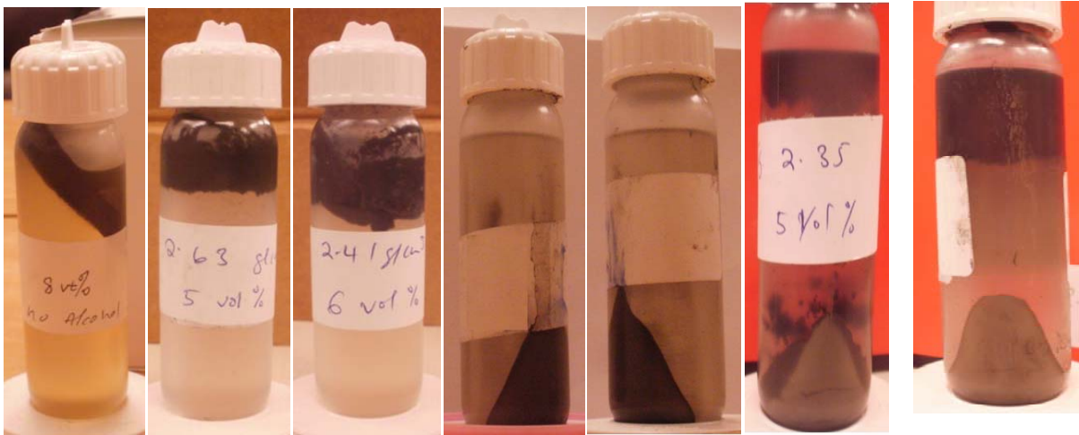
Fig.36 Centrifugation separation results with different heavy liquid (from left to right: (a) \rho_1=2.86 \text{ g/cm}^3 (b) \rho_2=2.63 \text{ g/cm}^3 (c) \rho_3=2.41 \text{ g/cm}^3 (d) \rho_4=2.08 \text{ g/cm}^3 (e) \rho_5=2.25 \text{ g/cm}^3 (f) \rho_6=2.35 \text{ g/cm}^3 , (g) \rho_7=2.37 \text{ g/cm}^3 )
