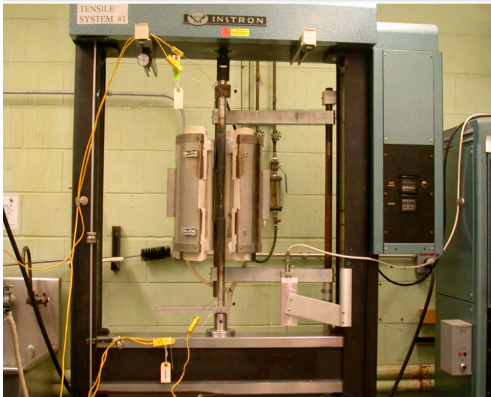
Figure 4. Experimental set-up of high temperature tensile testing.
