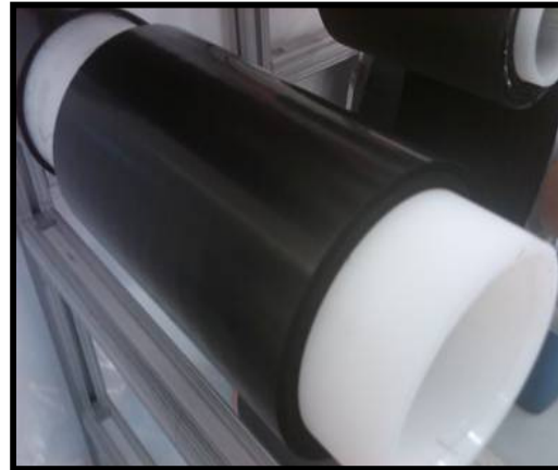
Figure 23B: the pilot coated 6” film of 2.0X M1X had excellent uniformity
