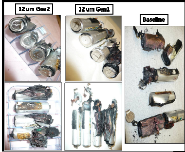
Figure 29A: cells after nail penetration test
