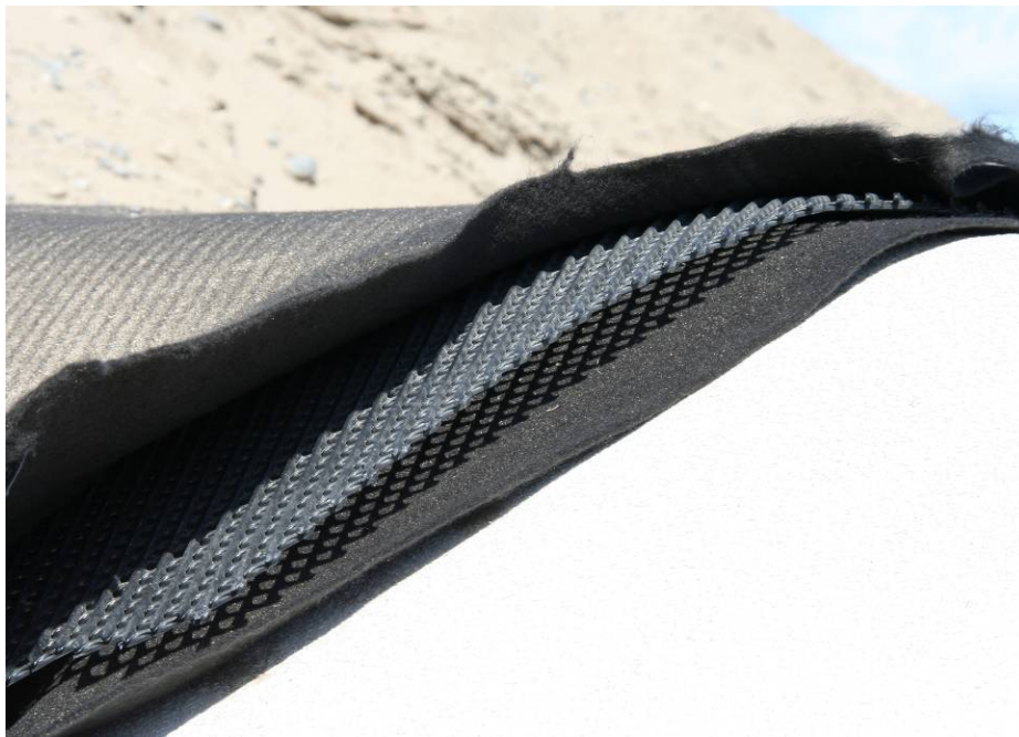
Figure 5. WCH Replaced a 12-in. Layer of Drainage Gravel with a Geocomposite Layer, Creating Space and Reducing Construction Cost.
