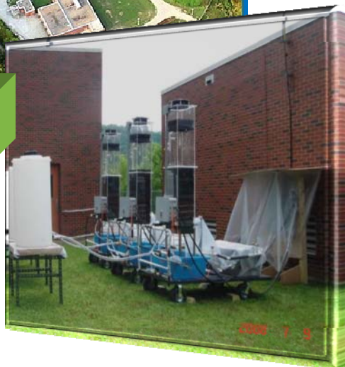
Pilot-scale cooling towers installed at FTMSA, PA
