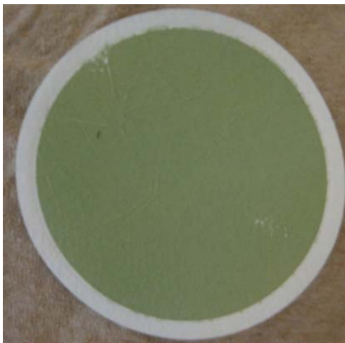
Figure 3.2.10 “Green deposits” retained on 0.45um filter paper after filtering the recirculating water in Tower B on day 9 in pilot scale tests with MWW_pH at pH 7.0
