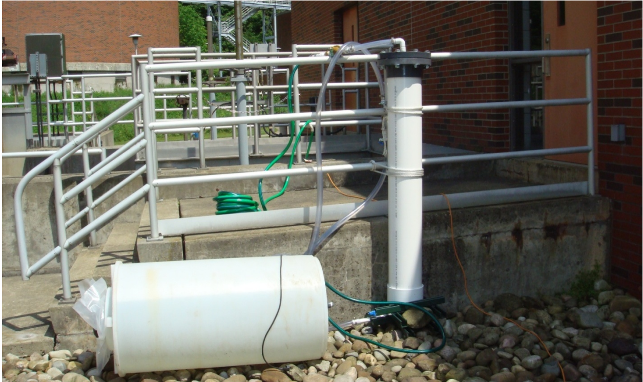
Figure C.6. Granular activated carbon adsorption column setup at FTMSA
