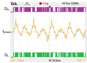
Fig.14 Phase current and change of duty cycle
