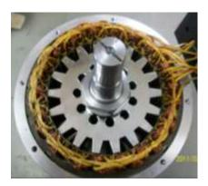
Figure 65: End of a Switched Reluctance Machine
