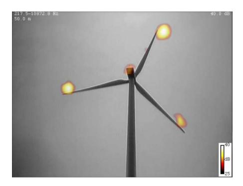
Figure 185: Beamform map of the GE 1.5 MW wind turbine using TIDY at a particular instant of time during its rotation.
