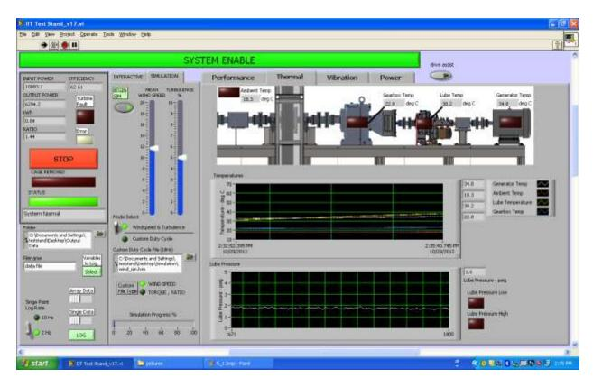
Figure 11Figure 11 and Figure 12 show screenshots of the software monitoring the Lab Field Unit regarding Performance, Thermal, Vibration, and Power.
