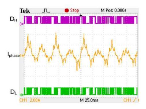
Figure 139: Phase current and change of duty cycle
