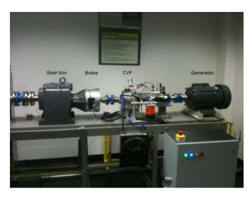
Figure 187: Viryd 8 kW wind turbine drive train simulator.
