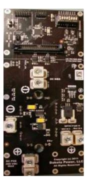
Figure 69: IGBT power driver board
