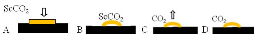
Figure 17. Proposed mechanism of blister formation. A. SCCO 2 diffuses into the coatings. B. SCCO 2 saturates the coating. C. CO 2 diffuses out of the coatings when pressure is reduced to atmospheric pressure. D. Remaining CO 2 changes into gaseous phase and causes blistering with extreme volume increase.
