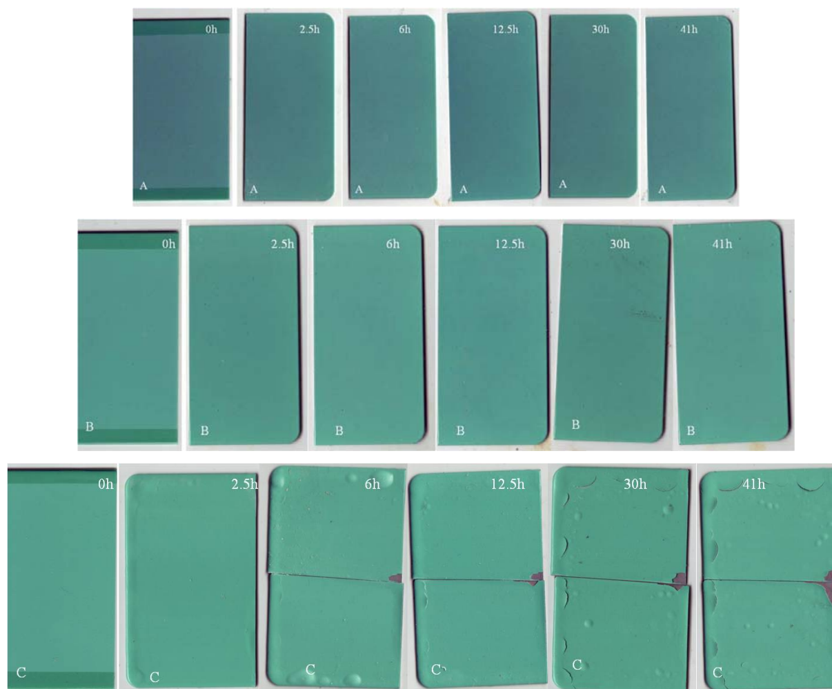
Figure 9. Coated panels with different exposure time to SCCO 2 of 32°C and 1100psi for 24 hours. A, S323-S-L, B, S323-S-M, and C, S323-S-H.
