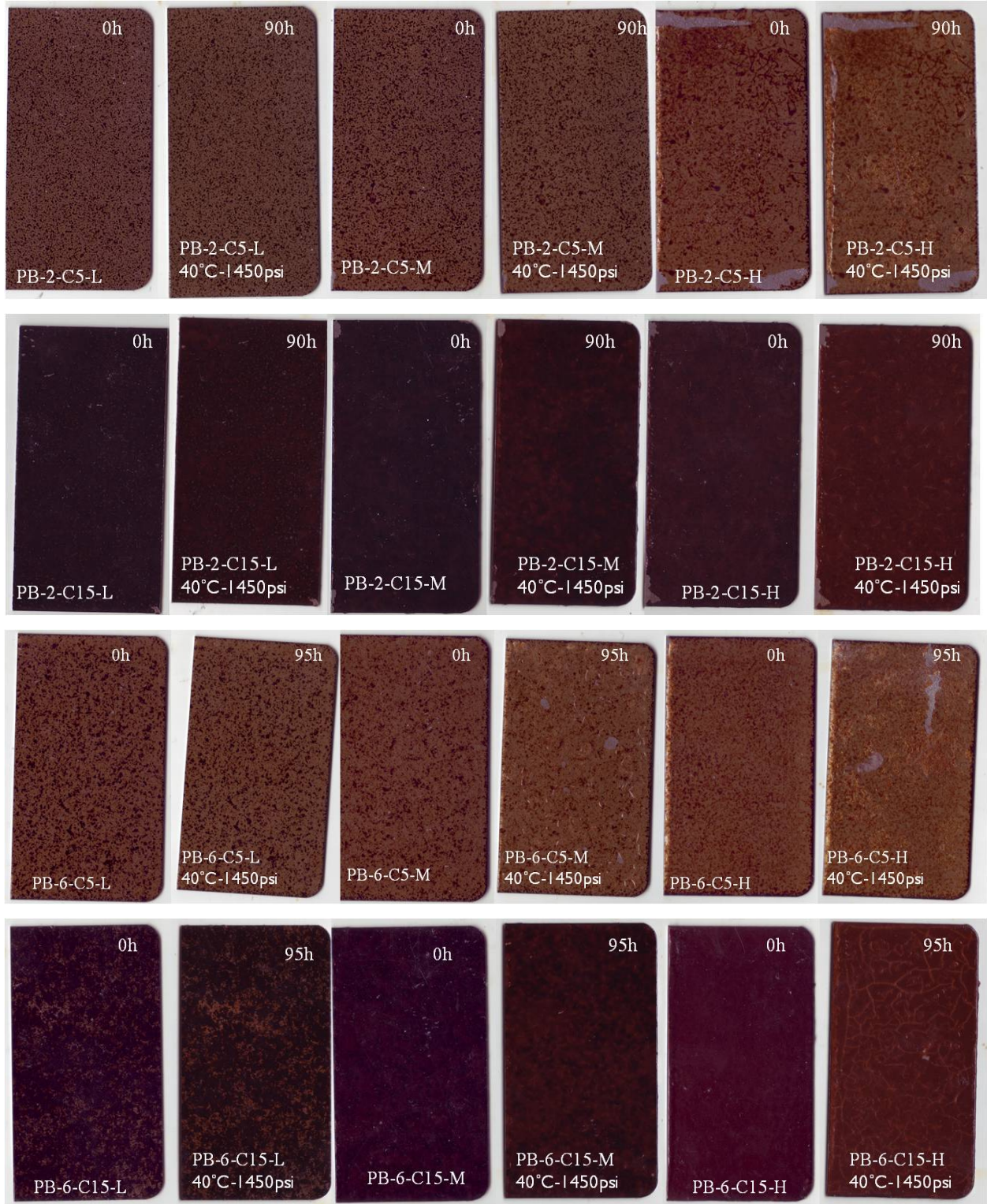
Figure 15. Coated panels with different exposure time to SCCO 2 .
