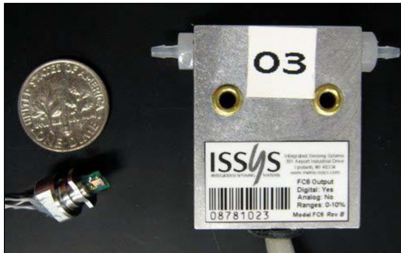
Figure 22 The ISSYS FC6 sensor shown at right with the Siargo TSC-2000 sensor at the lower left.
