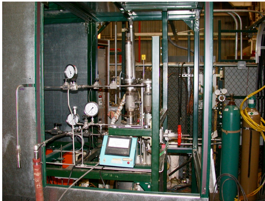
Figure 2-4. Forced convection sodium loop for materials testing.
