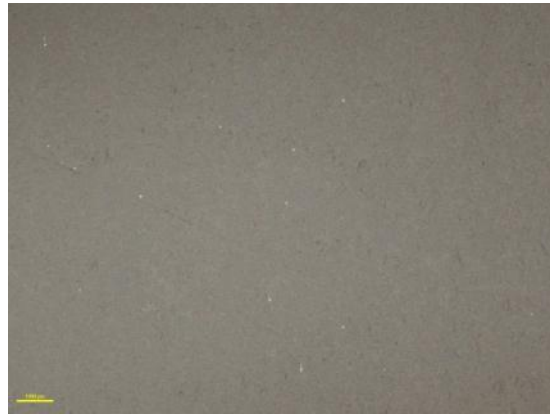
Figure 93. MPL surface morphology of the GDL made in production coating trial; the scale bar is 1 mm
