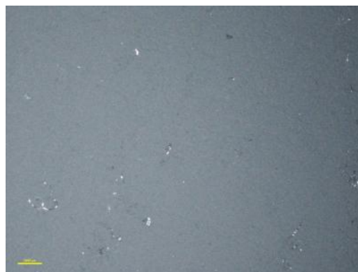
Figure 78. Surface quality of the MPL made from new ink approach and low HLB dispersant.
