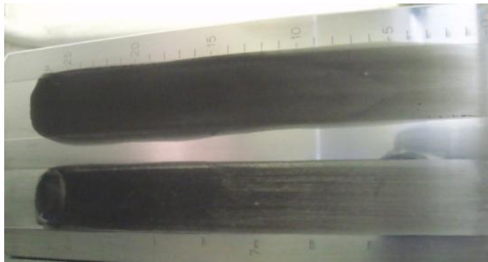
Figure 79. The cathode catalyst ink coated on the grind gage; Top: ink with filming and leveling control; bottom: same ink without filming and leveling control.
