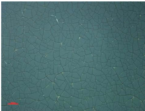
Figure 80. The surface quality of carbon paper 1 based cathode made with new formulation; scale-bar = 1mm.
