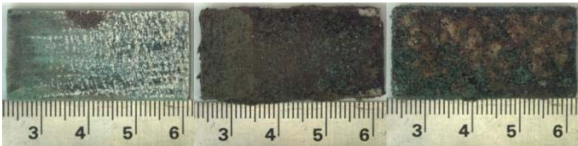
Left: 625 - 67% H 2 SO 4 67.5°C (2 nd test) Middle: 625 - 70% H 2 SO 4 85°C (1 st test) Right: 625 - 70% H 2 SO 4 85°C (2 nd test)
