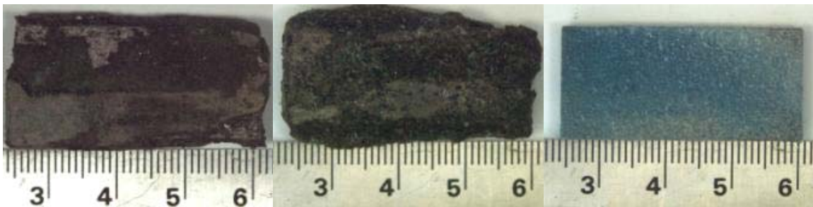
Left: 625 - 74% H 2 SO 4 115°C (1 st test) Middle: 625 - 74% H 2 SO 4 115°C (2 nd test) Right: 80% H 2 SO 4 150°C
