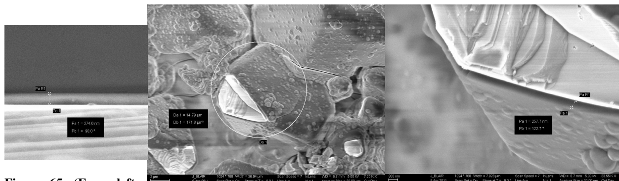
Figure 65. (From left to right): a) SEM of \text{Al}_2\text{O}_3 layer on Si control sample, 4b) SEM of cracked phosphor particle showing the deposition of a highly conformal coating of \text{Al}_2\text{O}_3 , ~ 260 nm thick, 4c) magnified view of a section of the phosphor showing a very conformal film in intimate contact with the phosphor material.
