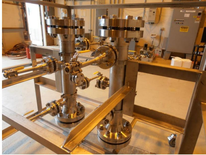
Figure II-36. The skid containing two pressure vessels in as-fabricated stage.
