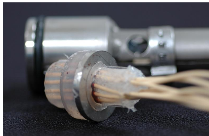
Figure A-63. Example of potted PBI-based hollow fibers.
