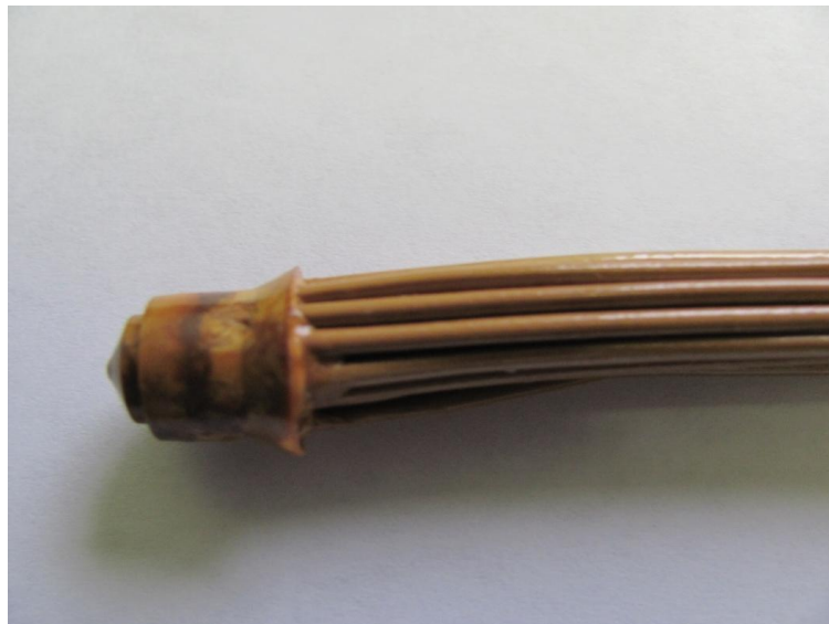
Figure II-25. Fiber bundle potted with PBI sealant.
