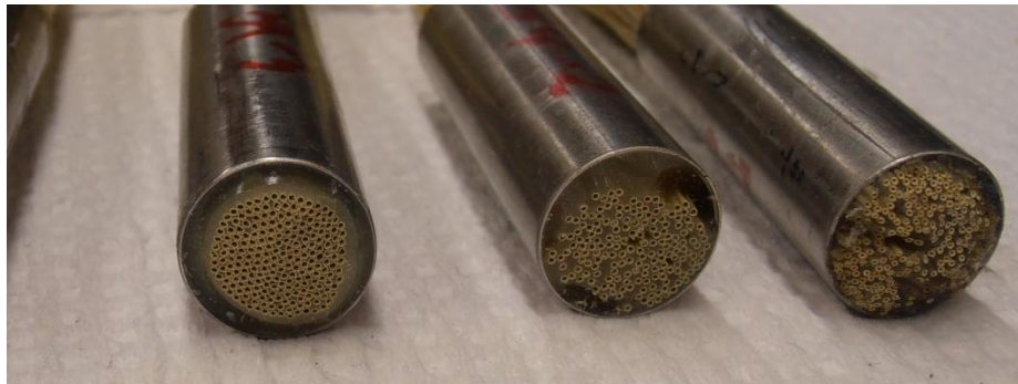
Figure II-27. Potted Fiber bundles assembled with varying packing densities to assess the potting performance
