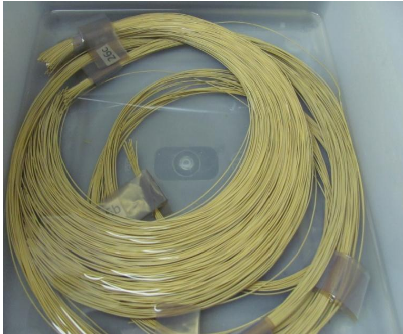
Figure II-23. Photograph of coils of 0.6mm diameter PBI hollow fibers fabricated at SRI.
