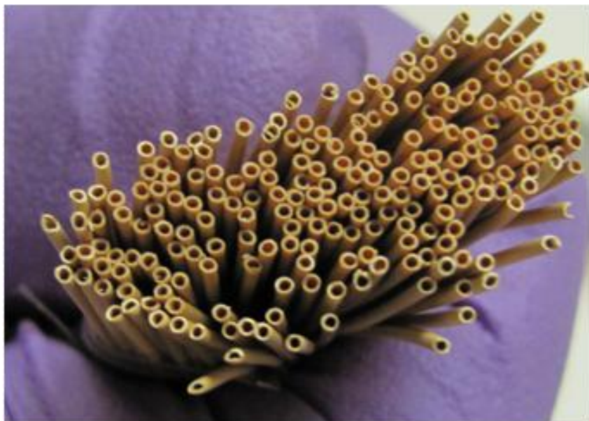
Figure II-21. A cross section of the PBI asymmetric hollow fiber made at SRI with no finger voids.
