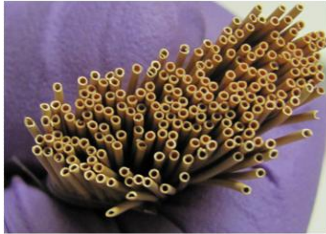
Figure E-2. Image of a bundle of PBI-based, asymmetric hollow fibers made at SRI.
