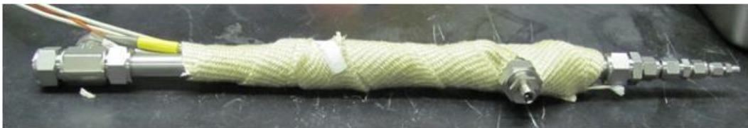
Figure II-32a. A photograph of assembled sub-scale 1-in module with SRI PBI hollow fiber membrane.
