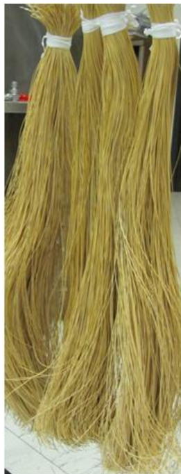
Figure II-16. A photograph of PBI hollow fiber bundles fabricated at SRI series B fiber.
