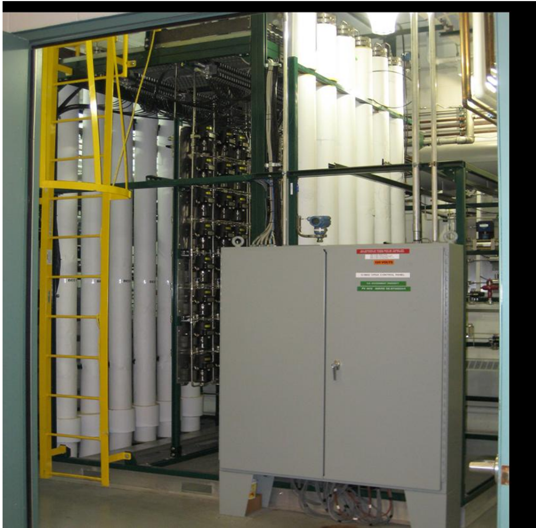
Figure 4.5 Photograph of the VPSA Continuous Operation Unit
