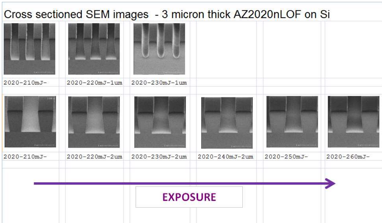
Figure 13A. Examples of acceptable profiles on AZ2020nLOF resist. Resist profiles are typically “box like”, with some slight undercutting at the base of the line. Notice that the lines are symmetrical.
