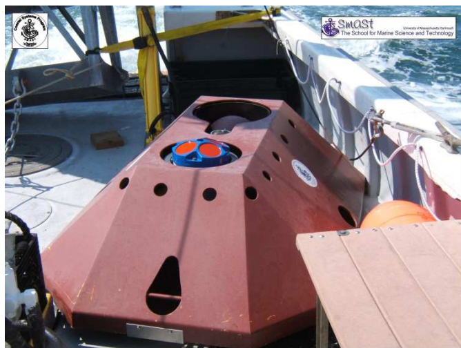
Figure 10: Bottom Mounted Upward Looking ADCP
