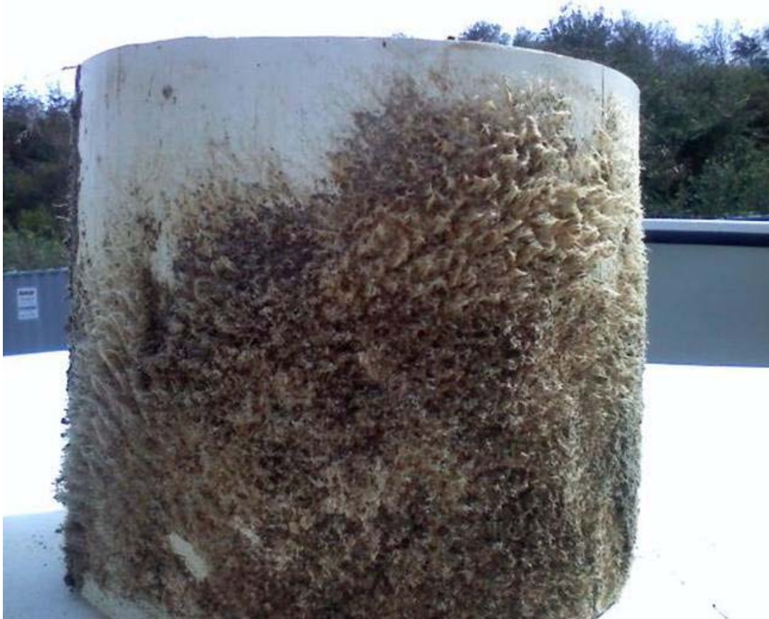
Figure 68 – Observed bio-accumulation on one of three un-treated fouling plates deployed in the high velocity zone of Muskeget Channel. The plate was positioned on the bio-fouling array to represent bio-fouling occurring in the upper portion of the water column. The bio-accumulation depicted resulted from being submerged for approximately 10 weeks.
