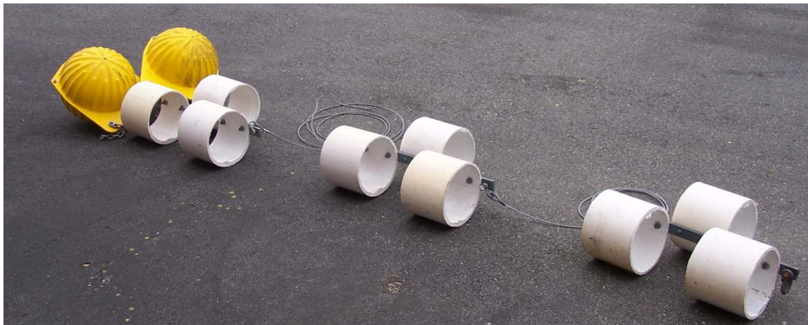
Figure 7 – Bio-fouling array (untreated) with three sets of fouling "plates" (surface, middle, bottom) arranged in triplicate for determining rate at which bio-fouling occurs on composite material utilized in the construction of a tidal turbine generating unit (ORPC OCGen Module).
