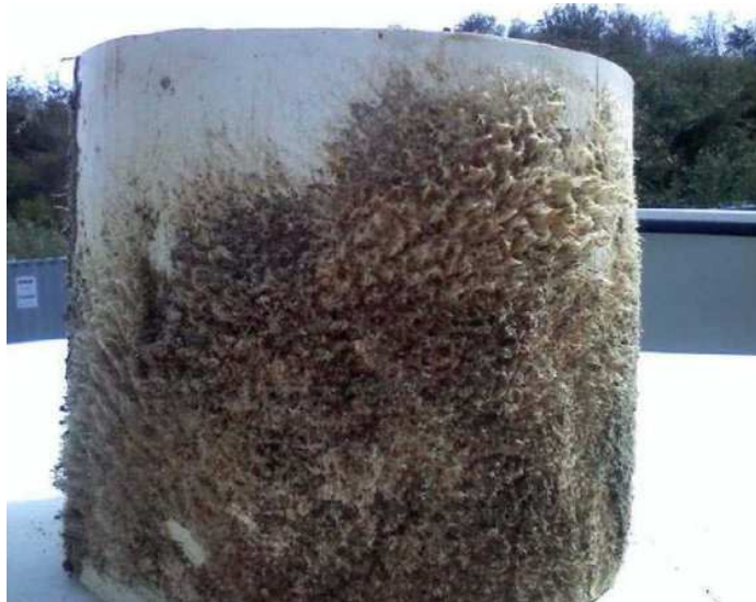
Figure 26: Untreated Composite Material Approximately Two Months After Deployment
