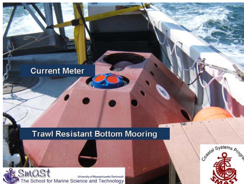
Figure 48 – ADCP deployed November 2010 to measure current velocity over a complete lunar cycle in the high velocity zone of Muskeget Channel.
