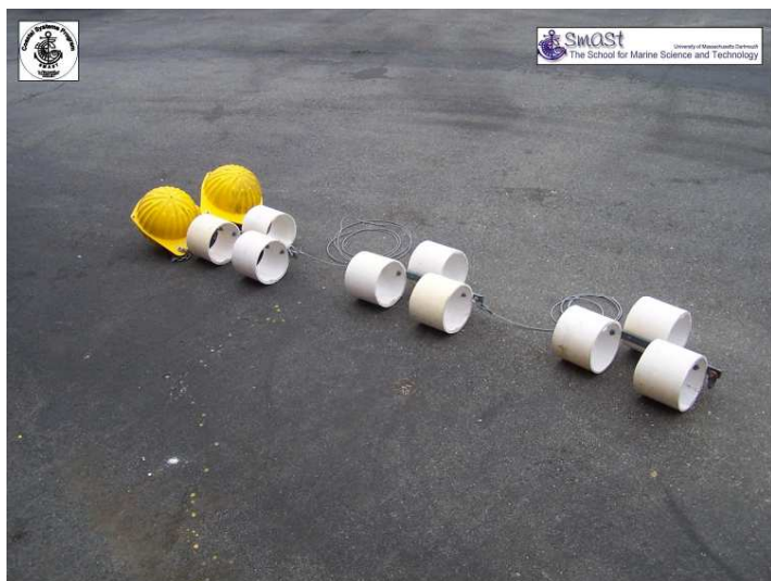
Figure 22: One of the Biofouling Arrays Prior to Deployment
