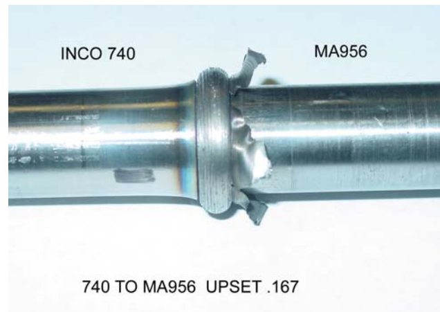
Figure 6. IN740-MA956 rod joints produced with material upsets in the 0.125" – 0.410" range.
