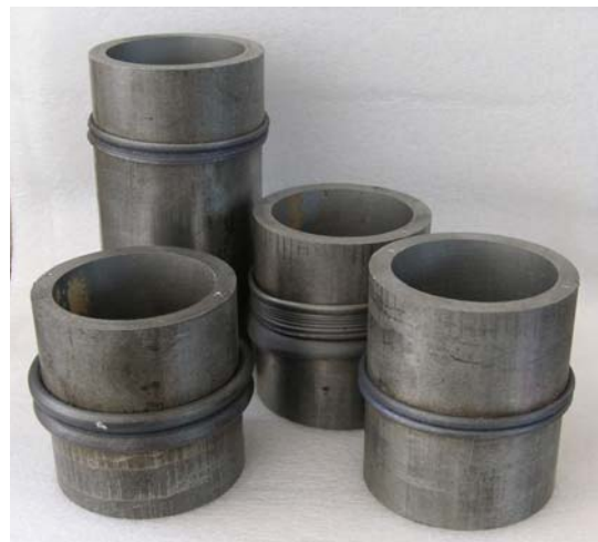
Figure 4. Typical MA956-MA956 butt welds produced under different welding conditions.
