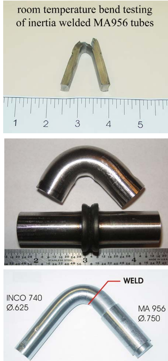
Figure 12. Room temperature three point bend tests in as-welded a) MA956-MA956, b) IN740-IN740 similar and c) IN740 – MA956 dissimilar joints.
