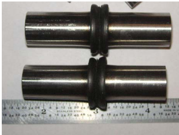
Figure 5. IN740-IN740 rod joints produced with material upsets in the 0.125" – 0.360" range.
