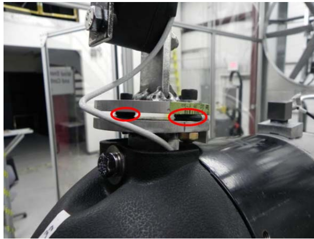
Figure 2-10: Rubber Grommets for Simulated Root Crack.
