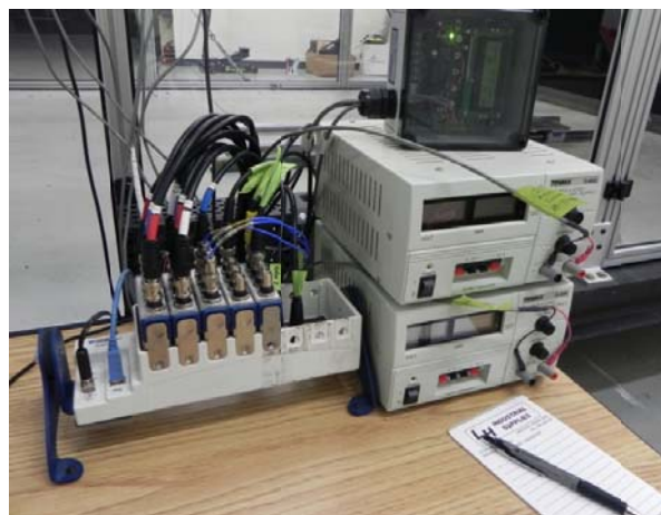
Figure 2-5: DAQ hardware, DC power supplies (2), and cup anemometer digital readout.
