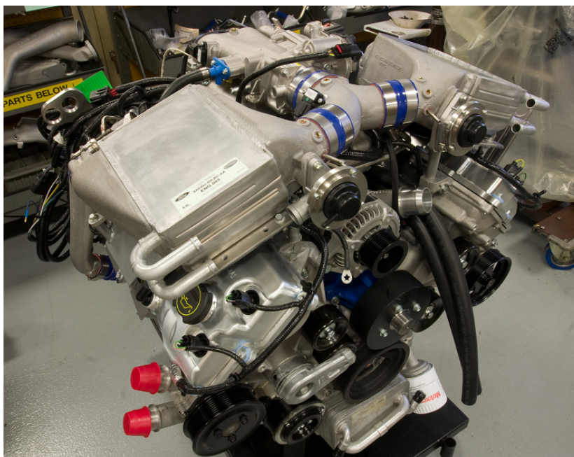
Figure 86 - Multi-cylinder engine with charge air coolers and throttle body installed.
