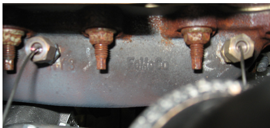
Figure 158 - Exhaust manifold with exhaust port thermocouples (cylinders 1 & 2).
