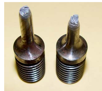
Hydrogen Testing - Faceted fracture surface with evidence for multiple secondary cracking
