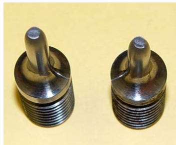
Helium Testing - Typical Ductile cup and cone fracture
