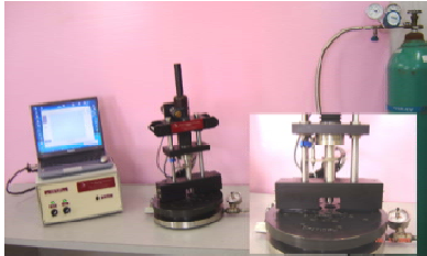
Fig. 1 – ATC SSM hydrogen testing apparatus. Picture on left shows set up, while picture on right shows details of pressurized hydrogen disk.
