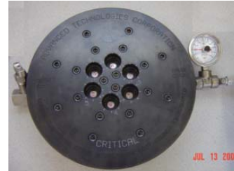
Fig. 1 – ATC SSM hydrogen testing apparatus. Picture on left shows set up, while picture on right shows details of pressurized hydrogen disk.
