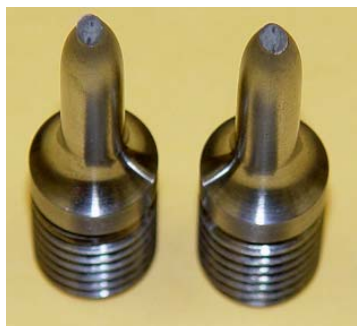
Helium Testing - Typical Ductile cup and cone fracture
