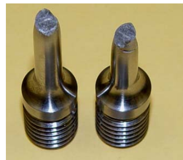
Hydrogen Testing - Faceted fracture surface with evidence for multiple secondary cracking, does not seem as severe as in Alloy A
