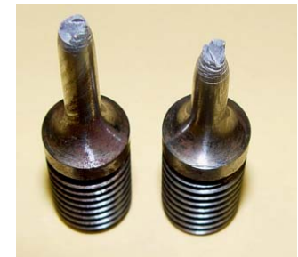
Hydrogen Testing - Faceted fracture surface with evidence for multiple secondary cracking
