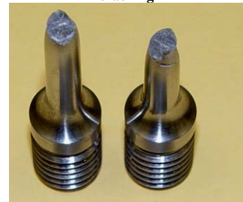
Hydrogen Testing - Faceted fracture surface with evidence for multiple secondary cracking, does not seem as severe as in Alloy A
