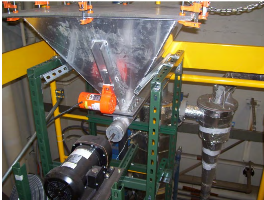
Figure 2: New vibrating screw coal feed system
