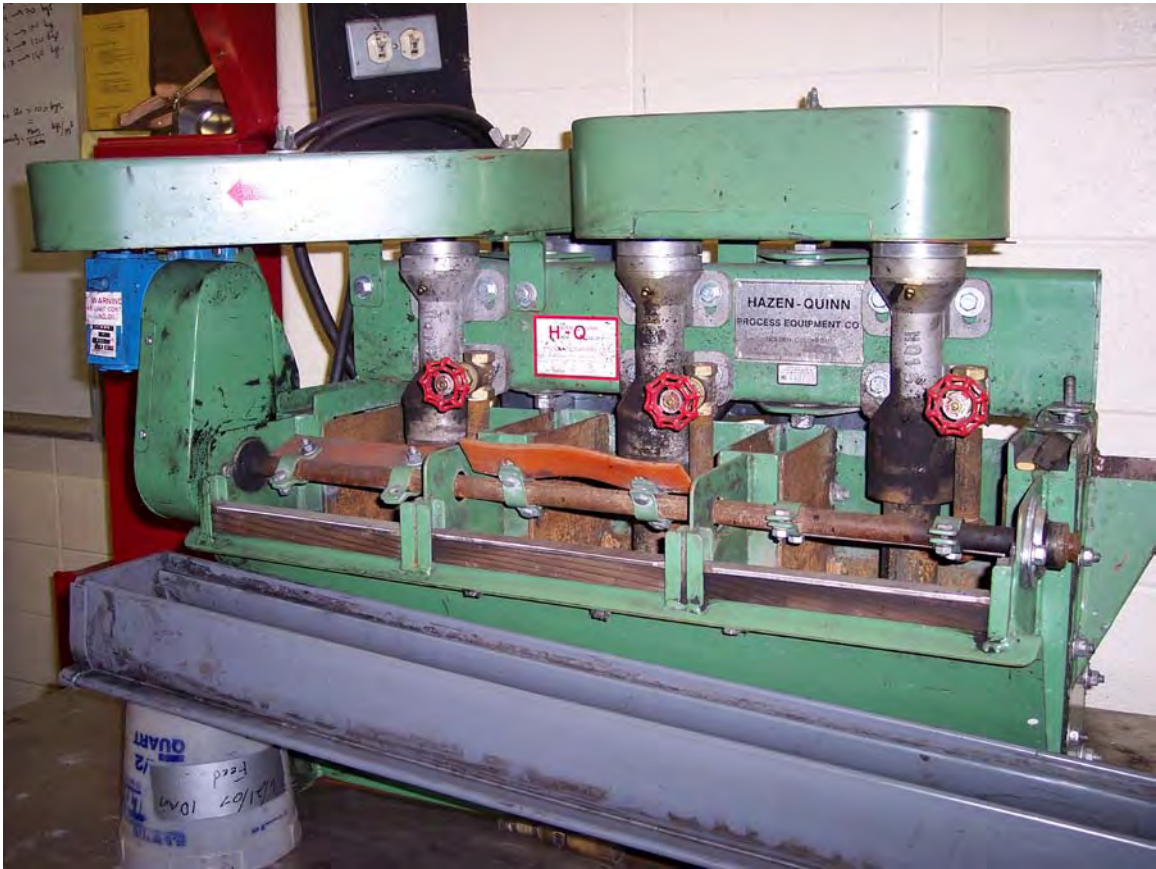
Figure 4. Conventional flotation bank cell used in plant with air eductor.
