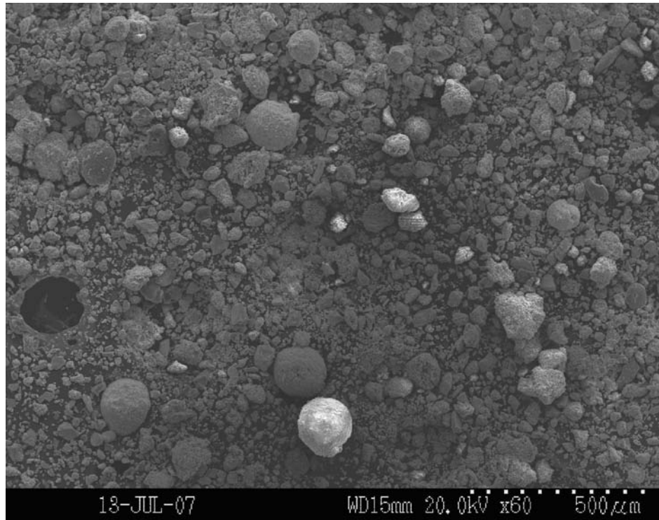
Figure 5. SEM picture of minus 177 \mu\text{m} particle size of magnetic plastic material at 500 \mu\text{m} optical resolution.
