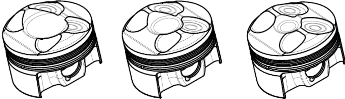
Figure 21:- Piston Designs To Support Compression Ratio Study (A) 12.5 : 1 (B) 13.5 : 1 (C) 14.5 : 1
