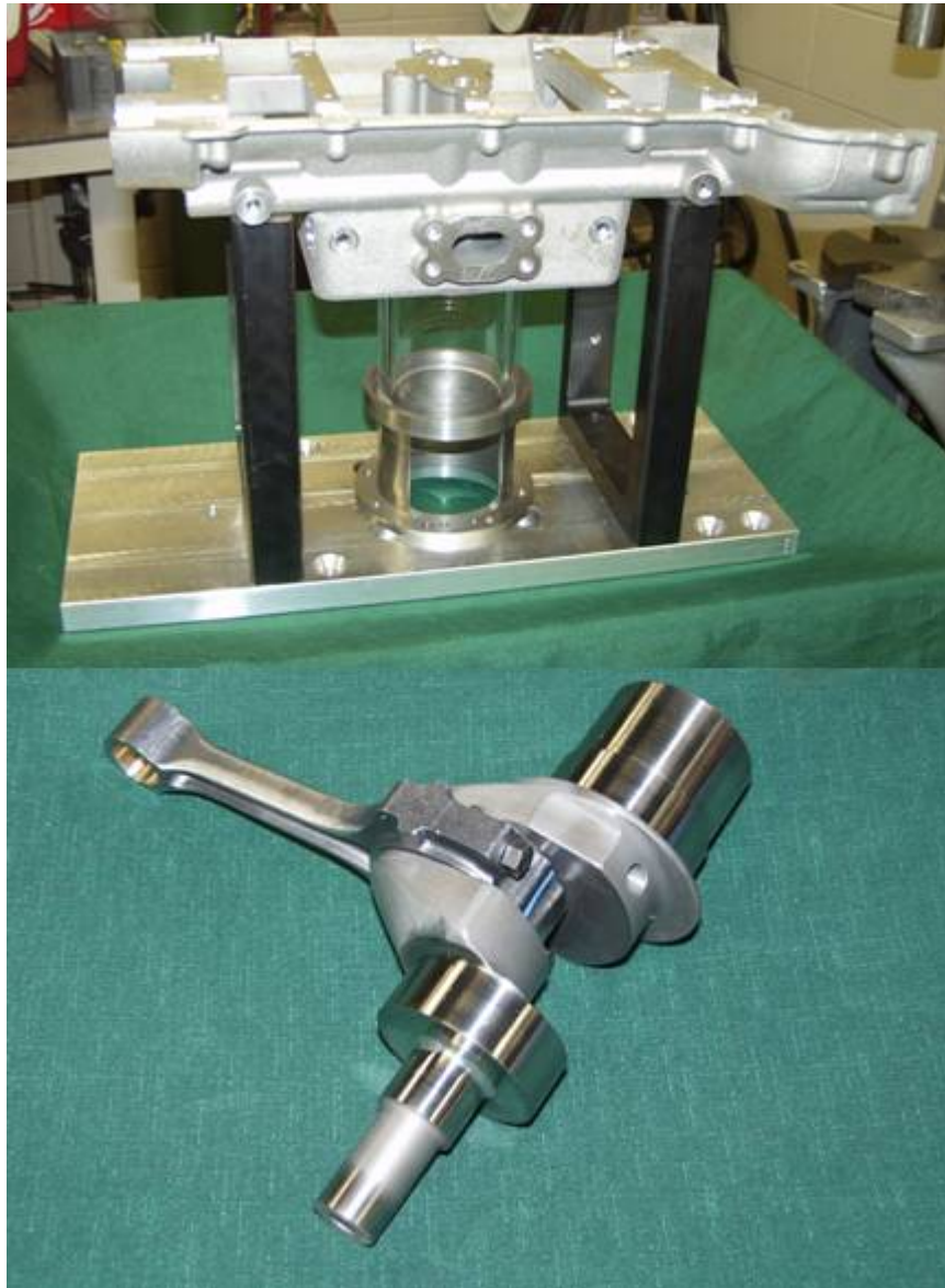
Figure 5:- Optical Engine Assembly Without Crankcase
