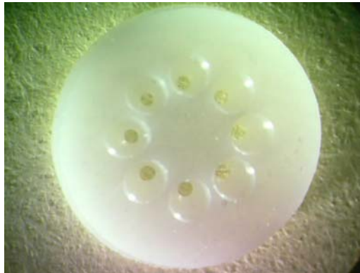
Figure 15:- Typical 8-Hole Nozzle Plate Configuration (Looking From The Outside Of Injector Tip)
