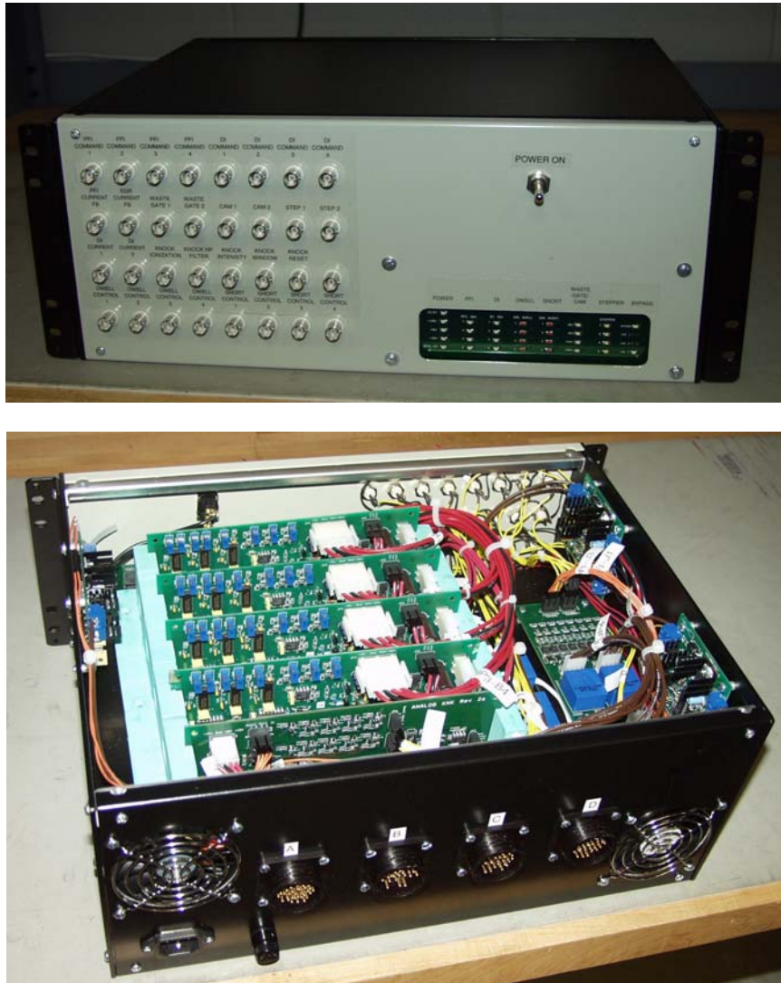
Figure 34:- Engine Control Interface, Including Ion Sensing Ignition System and LPDI Injector Driver
