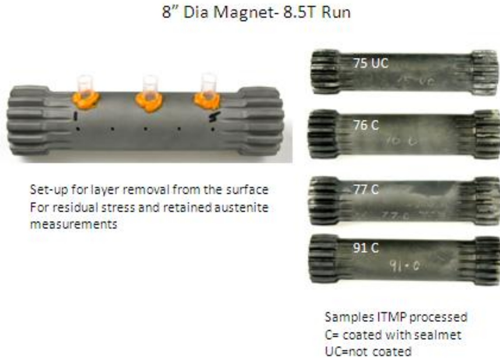
Figure 15: ITMP Orbital Drives with and without Coating
