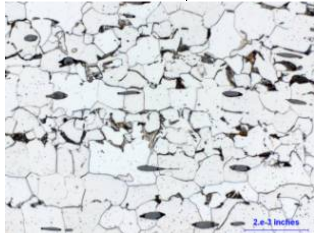
SAE1215 18T > T Curie @500X (30% ferrite increase)
