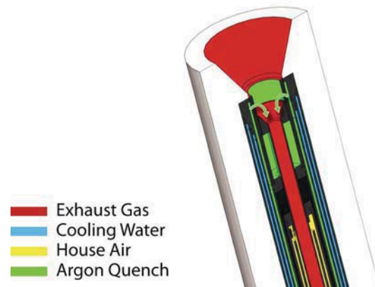
Figure 7. Schematic of extraction probe with flow channels highlighted.
